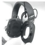
4. When placing the new ear pad, the halfround shape should be on top.
